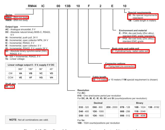
Figure 3.12: Decoding of the center encoder to understand its output data
