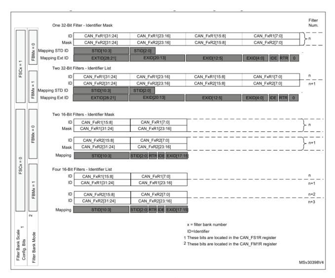
Figure 5.6: CAN filter registers
