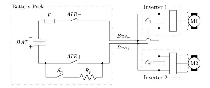
Figure 2.5: Logical diagram of the connection of the AIRs
