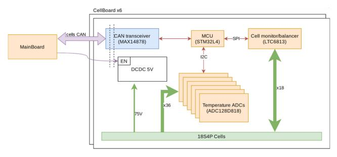
Figure 3.16: Structure of the BMS-HV
