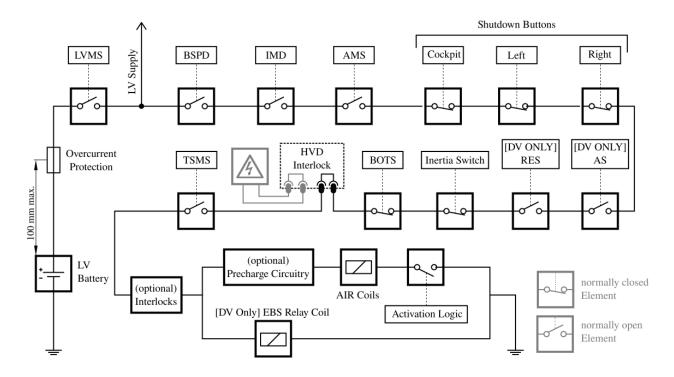
Figure 2.6: Shutdown circuitry
