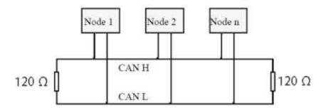
Figure 5.8: Can bus layout
