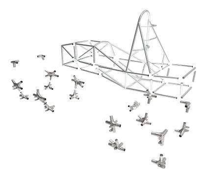
Figure 1.2: Chimera's chassis with 3D-printed steel joints
