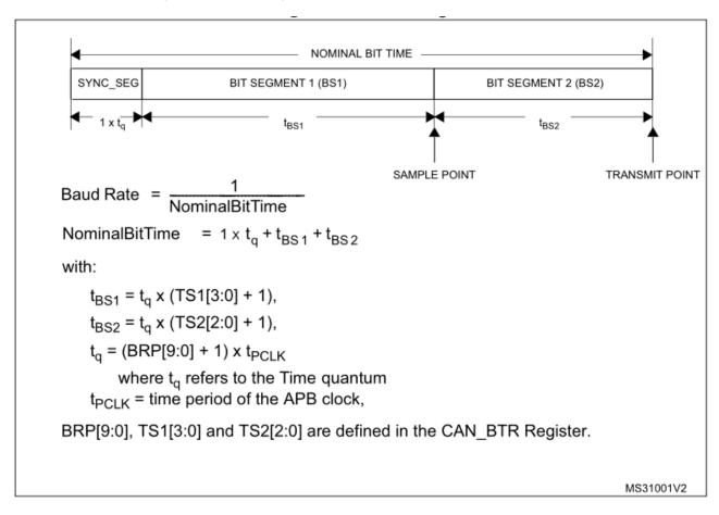
Figure 5.2: Subdivision of the nominal bit time into segments
