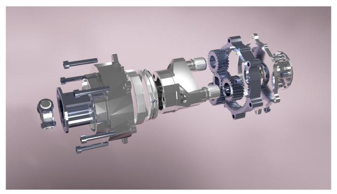
Figure 2.4: Planetary reduction gears
