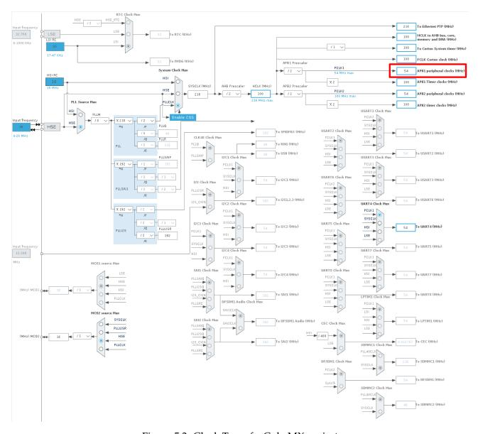
Figure 5.3: Clock Tree of a CubeMX project
