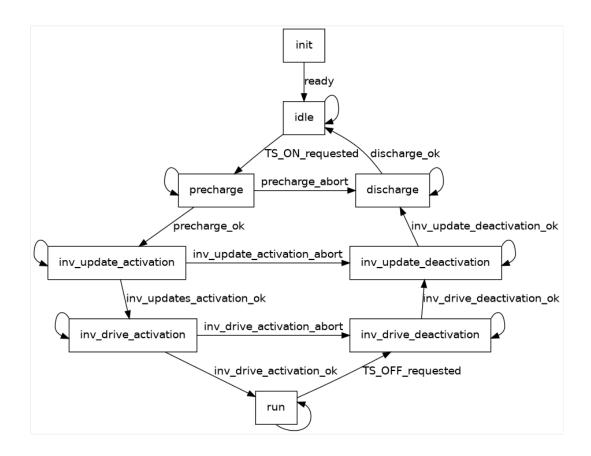
Figure 3.17: Flowchart of Fenice's FSM
