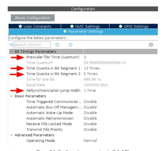
Figure 5.4: Configuration parameters in CubeMX
