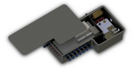
Figure 2.9: Render of the low voltage supply system
