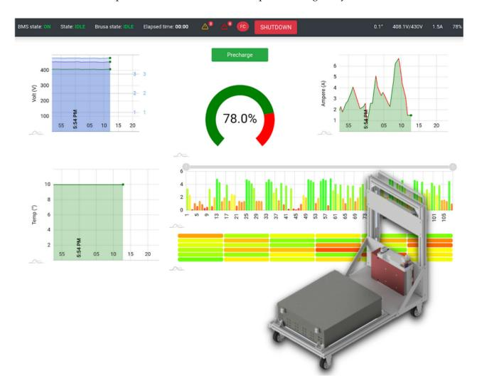
Figure 2.12: Render of the charging handcart overlayed to the web interface
