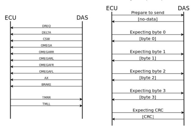
Figure 3.18: High-level and low-level representation of the Traction Control SPI protocol
