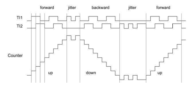
Figure 3.3: Example of a timer counter behavior in quadrature encoder mode.
