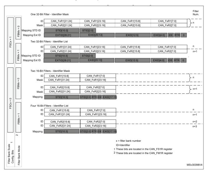
Figure 3.7: Layout and mapping of the bxCAN registers responsible for message filtering
