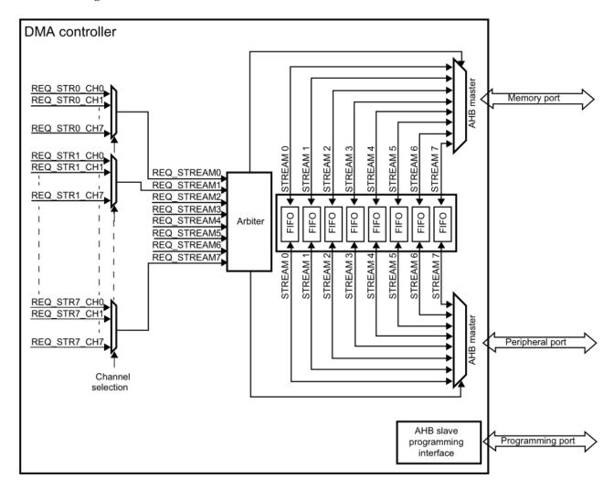
Figure 6.1: Block diagram of a DMA controller
