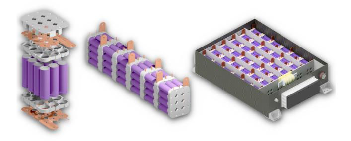
Figure 2.11: 3D models of one 3s4p module, one segment, and the complete battery pack
