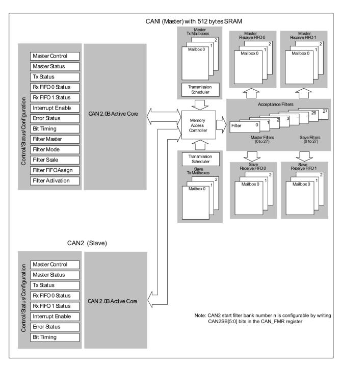
Figure 3.6: Block diagram of the bxCAN setup
