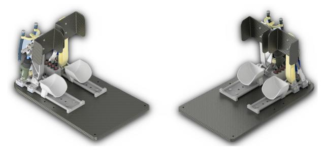
Figure 2.10: 3D model of the pedals assembly
