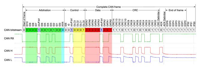
Figure 3.5: Example of the transmission of a CAN frame
