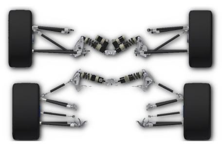
Figure 2.3: Suspension system of Fenice
