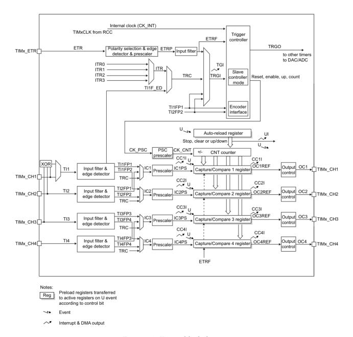
Figure 3.2: Timers block diagram
