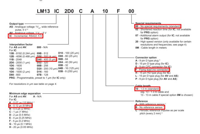
Figure 3.10: Decoding of the read-head part number to understand how to read its output signal
