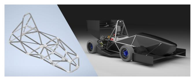
Figure 2.2: Render of Fenice and the tubular part of the chassis
