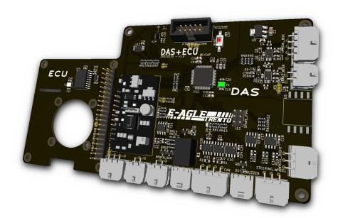
Figure 3.1: TECS PCB: on the left side, the 40-pin header to host the Raspberry Pi
